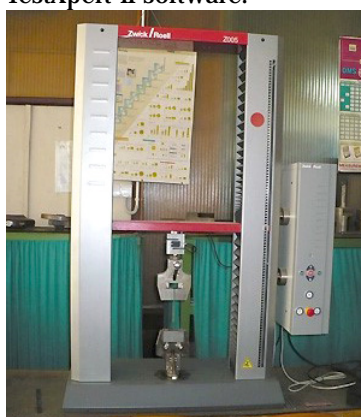
Fig. 7. Universal testing machine Zwick/Roell Z005
