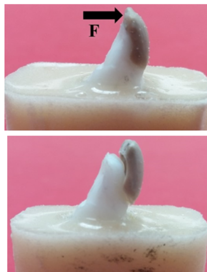
Fig. 8. The direction of the bending force applied to the incisal edge of the veneer (top) and its consequent detachment (bottom)
